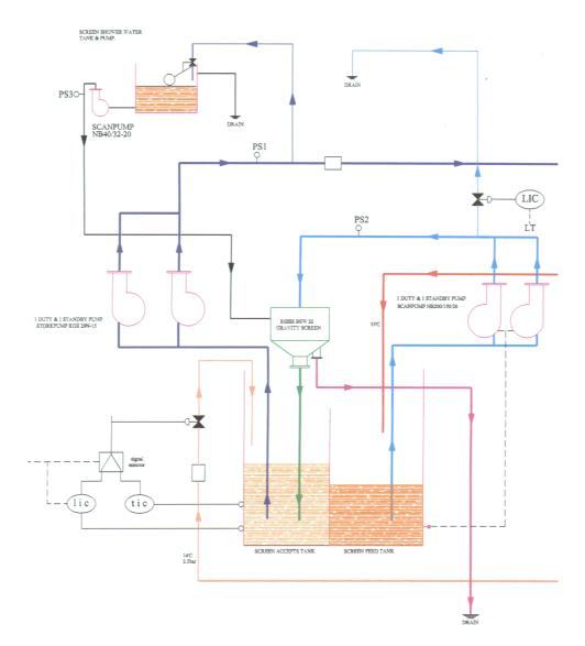
The design challenge was to ensure that appropriate pump impeller design and valve sizes were selected to obtain the specified operating points and dynamic performance. Of specific concern were the controllability of water temperature and levels in the two vessels within the plant. Traditional design methods concentrate on static operating conditions. However, *dynamic behaviour determines stability* and tests the physical limits of the plant.
